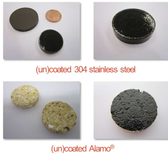
Figure 3: (Un)coated 304 stainless steel and (un)coated Alamo® refractory samples prepared for normal spectral emissivity measurements.
