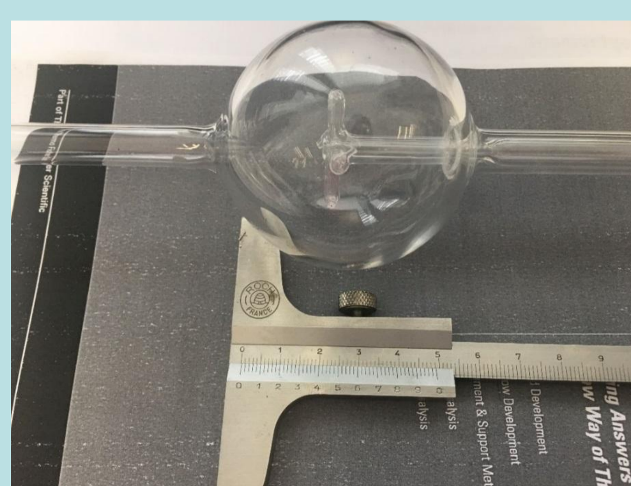
Fig. 2. The scale of jet stirred reactor
