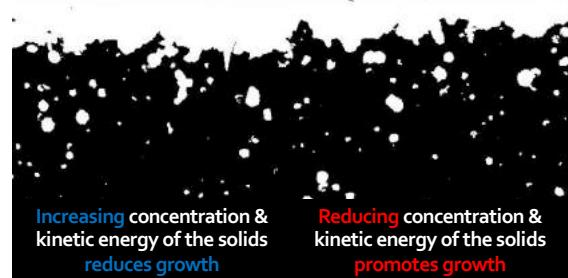
Increasing concentration & kinetic energy of the solids reduces growth
